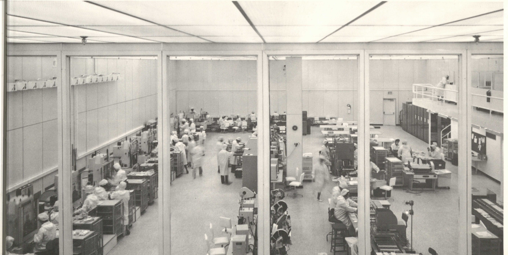
Franklin Mint proof quality coins and medals are minted in this special "clean room," where air is changed completely every 90 seconds. Personnel must wear lint-free uniforms, and anyone coming in contact with the coins must wear plastic gloves.
