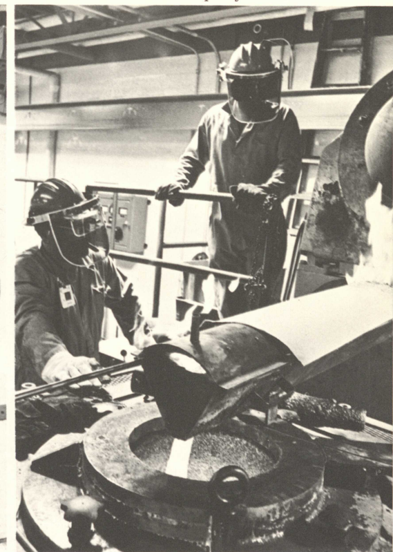
Automated continuous silver casting equipment, the first of its type in any mint, enables The Franklin Mint to melt, cast and roll millions of ounces of silver per year.
