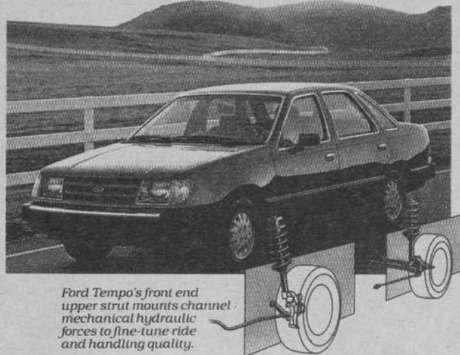
Ford Tempo's rear suspension longitudinal tie rods allow for "give" which reduces the effect of hard impacts.
