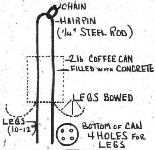
CUT THE STEEL RODS into 5-foot lengths. Bend the 5-foot pieces around a 1-inch pipe to shape them into hairpins as illustrated. You will use two of these hairpins for each anchor. Slip the straight leg of the hairpin through the loop at the end of your 6-foot chain and pull the chain loop up to the bend in the steel rods.
