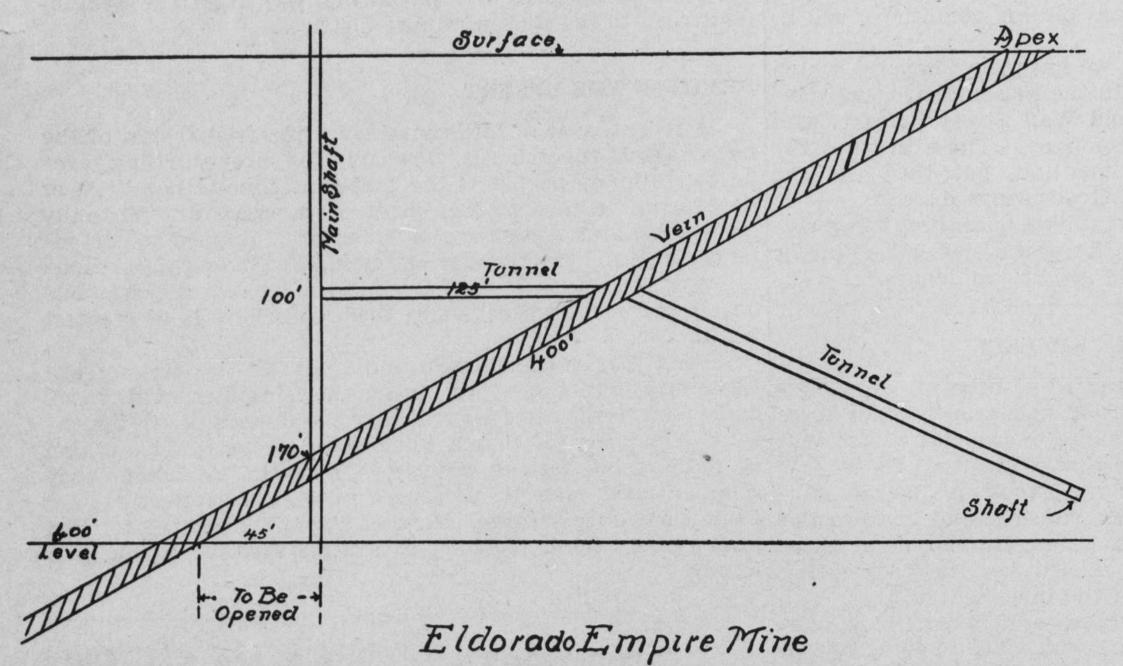
Main North-South ore-filled fracture along Major Fault that cuts across Eldorado Canyon and which may be the Mother Lode of all the East-West veins shown on first sketch. A fifty-foot drift now to be driven will open all veins at the 400-foot inclined level where rich strikes are possible.
