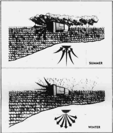
The high efficiency heat pump saves energy because it uses existing heat. In the winter it moves heat found outside to inside your home. In the summer the process is reversed.
