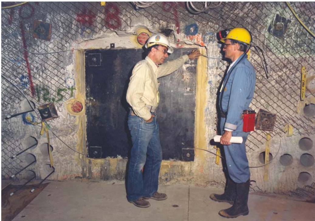
Photo 18: Francois Heuze, LLNL, and Les Hill, SNL, discuss details of the CONVEX plate experiment that is to the left. The cavity wall behind contains ports for gauges and rock bolts.
