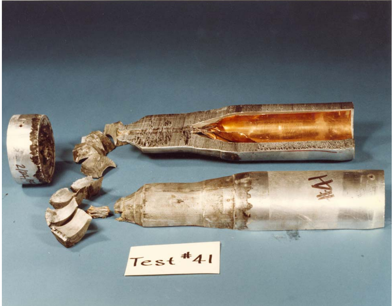
Photo 5: A tenth-scale closed FAC model—longitudinal cross section. The anticipated weak section was notched to produce an ogive shape. Pieces were glued back into position to match shock impedances along the closure section.
