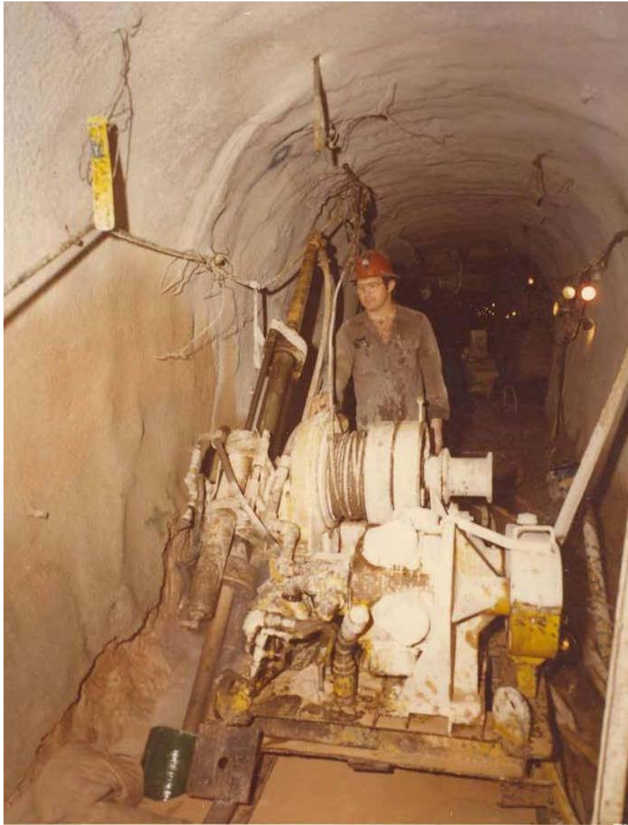
12 – John F. Campbell next to a Diamond Drill Rig in U12N Tunnel
